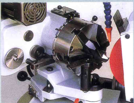
◀ Grinding Conventional point drill
